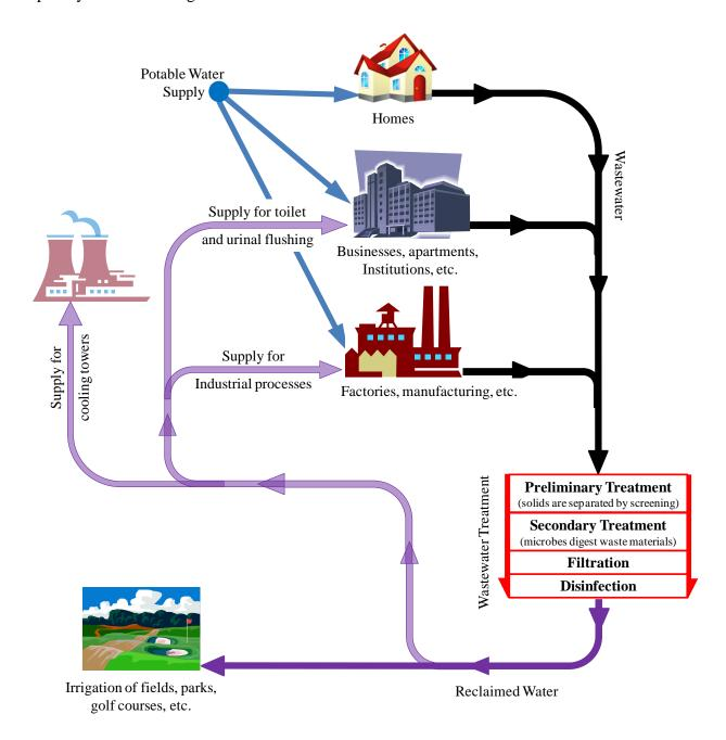
While reclaimed water typically looks like potable water, it is not treated to potable water standards. The urban water reuse standards for Georgia are established in the Georgia EPD Guidelines for Water Reclamation and Urban Water Reuse and are as follows:
